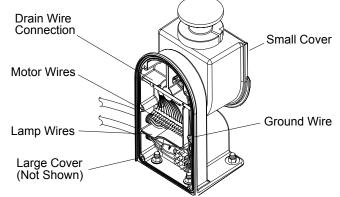
13. Reinstall large cover on remote mounting assembly ensuring tight seal.
