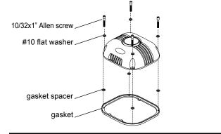
Note: Ensure #10 washers and gasket spacers are installed as pictured above.
