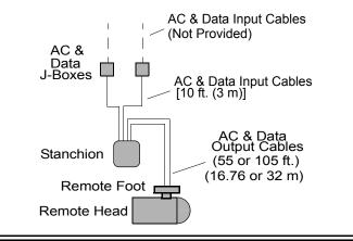
CAUTION: This equipment contains sensitive electronic components that require electrical isolation during installation and operation. DO NOT arc weld on mounting platform with electronics assembly installed in luminaire stanchion.
